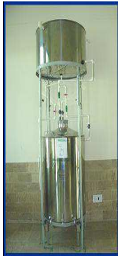
Figure 6. Schematic view of 300 liters arsenic removal unit (ART), showing various components
