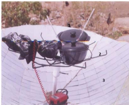
Figure 1. Experimental set-up of parabolic dish multi-solar cooker; 1-pot; 2-pot holder; 3-reflector.
