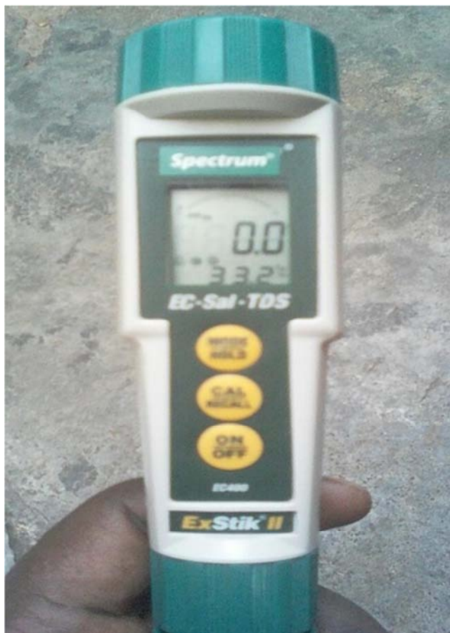
Figure 3. Spectrum® Waterproof Electric Conductivity Meter Used for Physicochemical Analysis.
