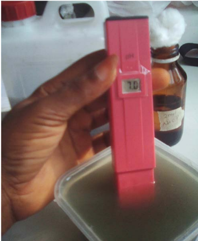
Figure 1. Adjustment of pH of the tannery effluent to neutral prior to bioremediation.
