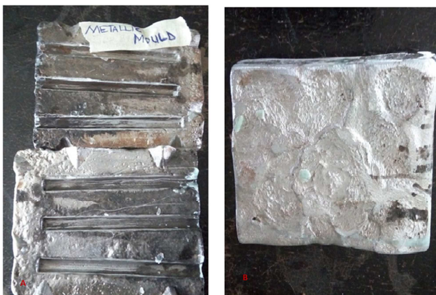
Figure 1. Mould for the inlay wax: (A) open; (B): closed.
