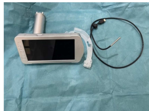
Figure 3. Quick Air device, curved blade and cable.
