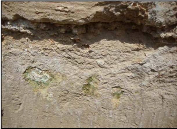
Figure 22. Shows the growth of algae on the external surface of one of the limestone' coffins.
