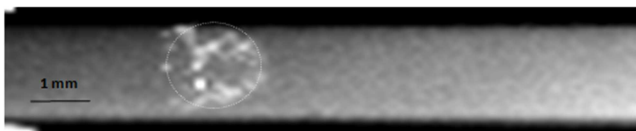
Figure 6. Image of the dynamic observed in an experimental system of a nitrogen gas bubble (center; left end), releasing into a column filled of medium crude oil of 25 °API at a constant temperature of 150°C, and pressure of 5950 psi (Reservoir Studies Management Laboratory Gas Injection IOR, 2016).
