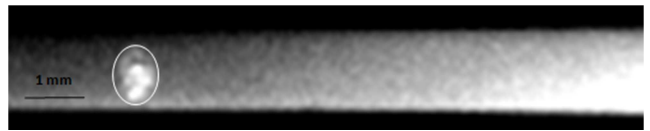
Figure 8. Image of the dynamic observed in an experimental system of a nitrogen gas bubble (center; left end), releasing into a column filled of medium crude oil of 25 °API at a constant temperature of 150°C and P value of 7000 psi (Reservoir Studies Management Laboratory Gas Injection IOR, 2016).
