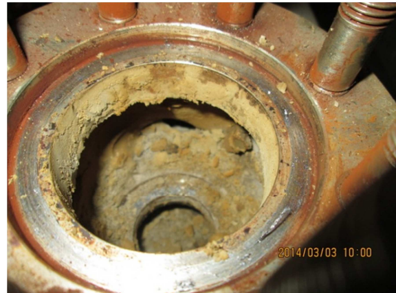
Figure 4. Ammonia injection control valve cover before cleaning.
