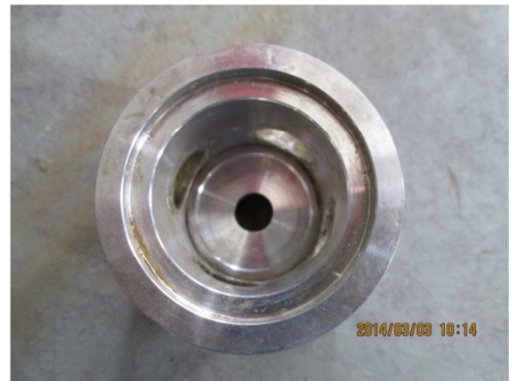
Figure 5. Ammonia injection control valve cover after cleaning.
