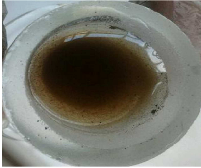
Figure 3. Khaki blockage dissolved in water.
