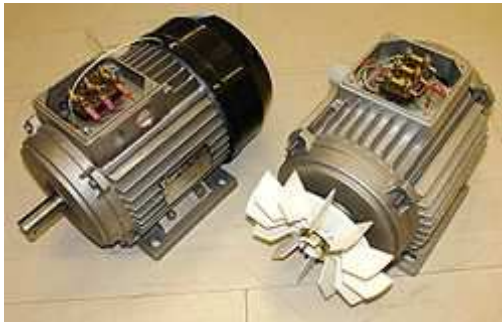
Figure 1. Three-phase totally enclosed fan-cooled (TEFC) induction motor, with and, at right, without end cover to show cooling fan. In TEFC motors, interior losses are dissipated indirectly through enclosure fins mostly by forced air convection
