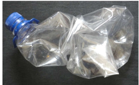
Figure 3. Demonstration of high permeability of hydrogen gas: PET bottle with gaseous hydrogen 4 weeks after filling [3]. Gaseous oxygen does not have such penetration.
