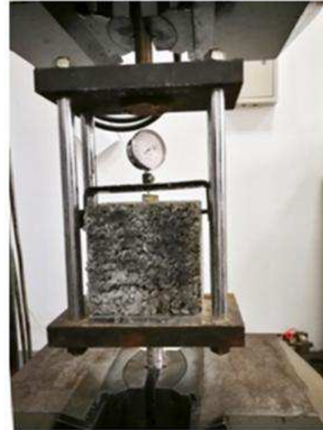
Figure 4. Bonding force test between permeable concrete and bolt.
