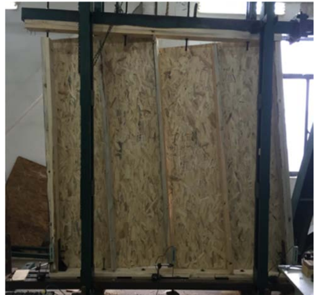
Figure 8. Failure of the shear walls.
