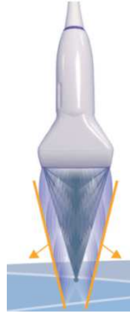
Figure 4. Shear wave amplification and enhancement based on the principle of Mach waves (orange lines).
