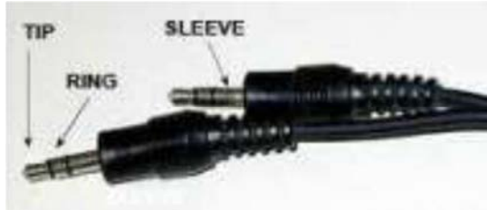
Figure 17. Different sections of audio cord terminal.
