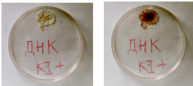
Figure 1. This Is a Drop of 0.1 M KI Solution Containing DNA, Immediately after Drying (Left) and after 24 Hours after Drying (Right). Drying Occurred at a Temperature of 20 – 22 C. (ДНК Is DNA in Russian).
