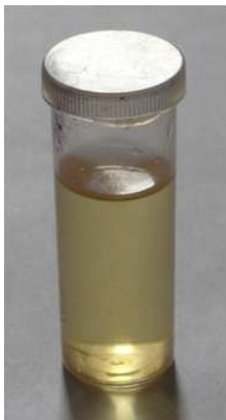
Figure 2. The Resulting Reaction Solution Containing Components of the Reaction Mixture, Which Are in Dynamic Equilibrium: 2KI + H_2O_2 (H_2O + O^*) \leftrightarrow I_2 + 2KOH . The Reaction Solution is Initially Slightly Yellow.
