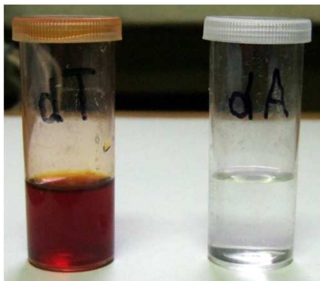
Figure 3. The Solution Containing the Reaction Mixture: 2KI + H_2O_2 (H_2O + O^*) \leftrightarrow I_2 + 2KOH , Was Originally Pale Yellow, in ~30 Minutes Became Brown in the Presence of a Few Crystals of TMP (Left), Whereas it Became Colourless in the Presence of a Few Crystals of dAMP (Right).
