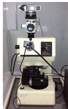
Figure 5. Dynamic hardness tester.
