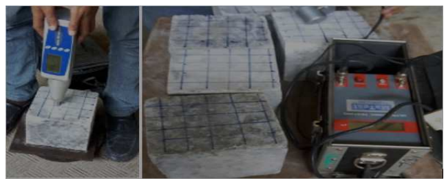
Figure 6. For Schmidt rebound hammer and ultrasonic pulse velocity testing at 56 th day.
