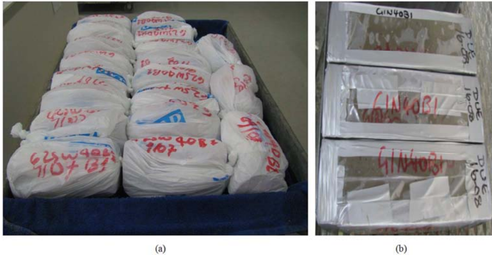
Figure 1. Curing of geopolymer concrete specimens (a) cylinders (b) flexural beams.
