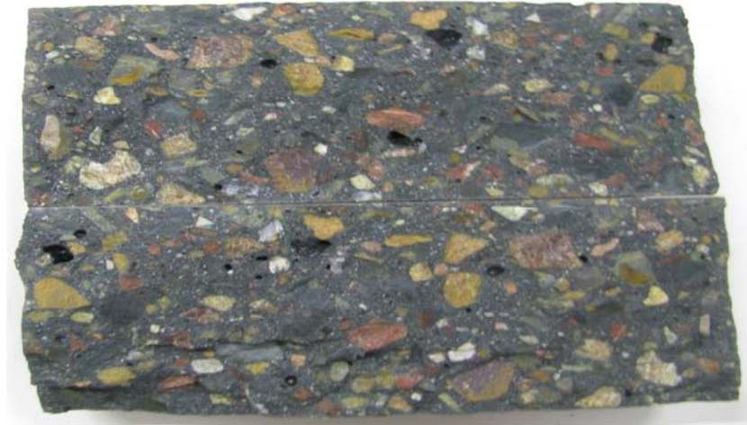
Figure 3. Fracture surface of hardened high-strength geopolymer concrete.
