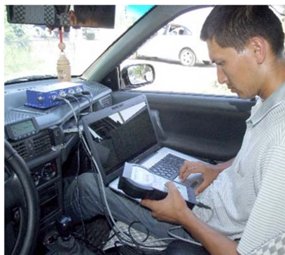
Figure 7. Installation and data collection with roughometer III.
