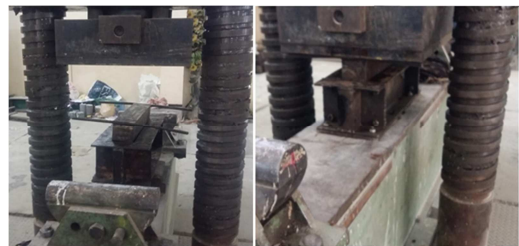
Figure 3. Compaction process of the mold.
