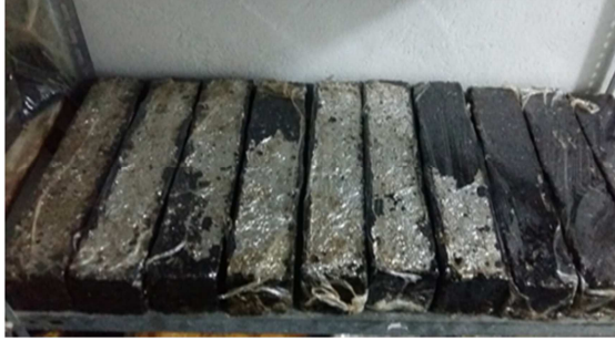
Figure 5. Part of the prepared beam specimens.
