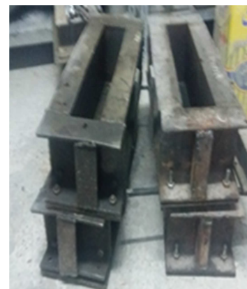
Figure 4. The casting molds.
