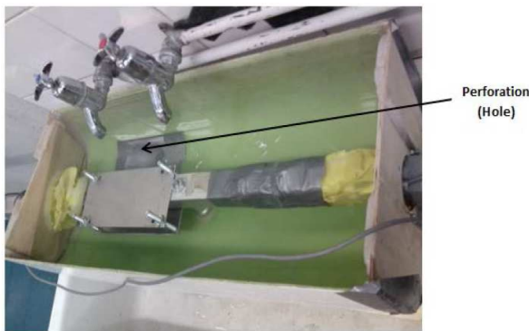
Figure 2.3. Damaged segment of ship model.
