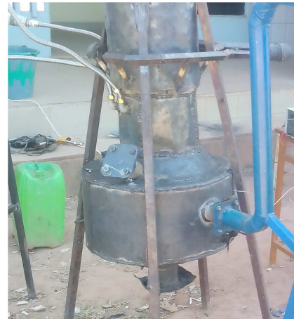
Figure 7. Downdraft gasifier with the water vapor generation circuit.
