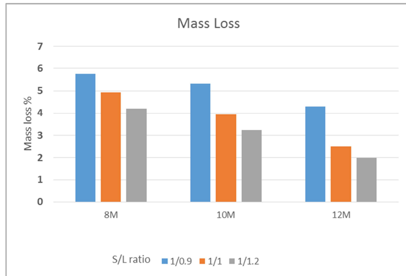
Figure 6. Mass loss of fly ash geopolymer mortars after 25 days of submersion in 2% H_2SO_4 .
