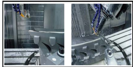
Figure 2. The surfacing operations (side 1 and 2) by copying cutter \Phi 50 .
