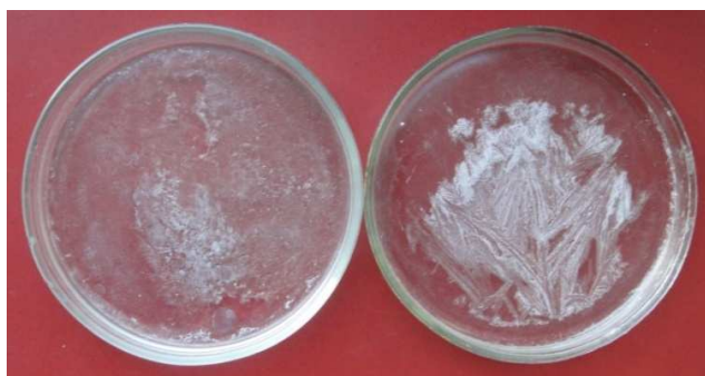
Figure 4. Such crystals were formed after drying of solutions from the anode (left) and cathodic (right) compartments of the operating electrolyzer, initially filled with a \text{K}_2\text{CO}_3 solution.
