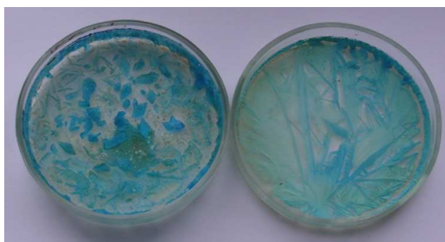
Figure 3. Such crystals were formed after drying of solutions from the anode (left) and cathodic (right) compartments of the operating electrolyzer, initially filled with a \text{CuSO}_4 solution.
