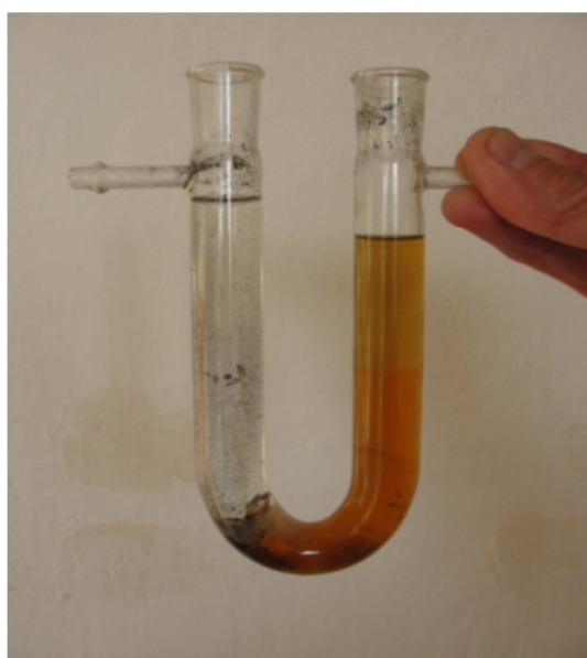
Figure 2. This is the result of electrolysis of blood diluted with 0.1 M NaCl solution (1/100) in an electrolyzer without a membrane.
