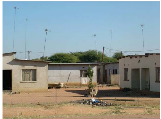
Figure 3. Typical buildings in developing countries with ungrounded metal roofs and metal protrusions such as television antennas. In the event of a lightning strike to the roof or protrusion it is highly possible that a side flash (or multiple side flashes) will leap to the body of occupants of such shelters.
