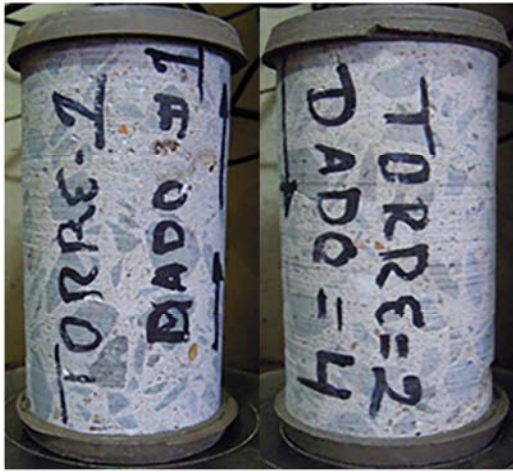
Figure 1. Cores extracted from two electric transmission towers.
