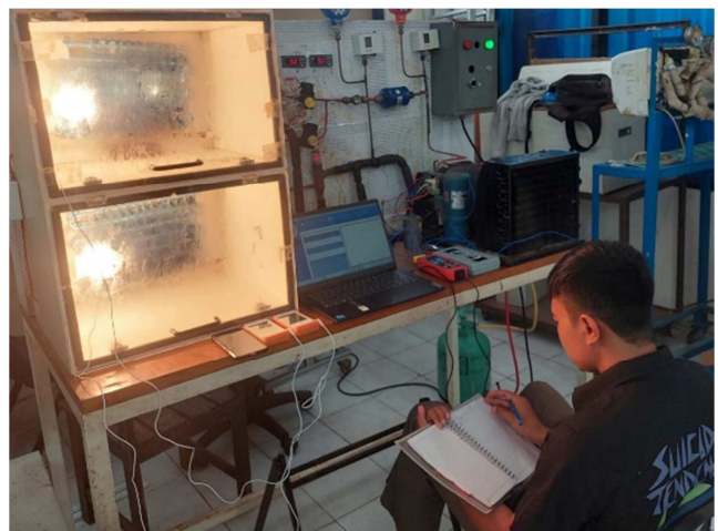
Figure 4. Basic refrigerator simulation machine testing process with two evaporators.
