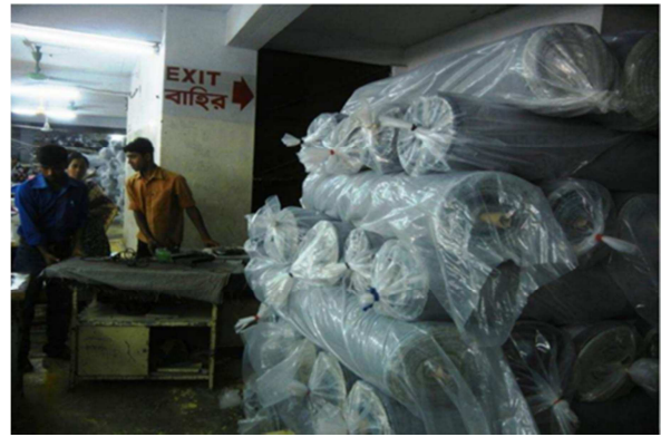
Figure 6. Soft factors: The exit gate meets as per regulation but is blocked [24].
