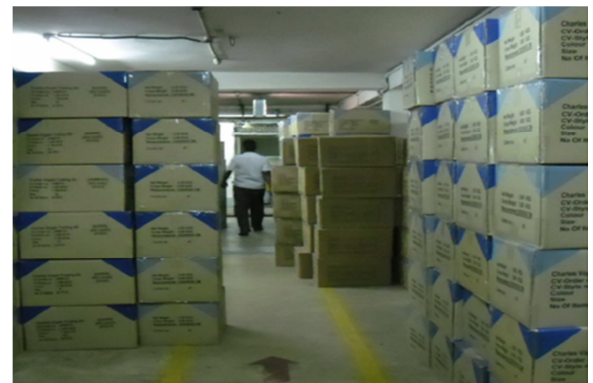
Figure 7. Soft factors: The exit corridor width meets regulation but is reduced in practice [24].
