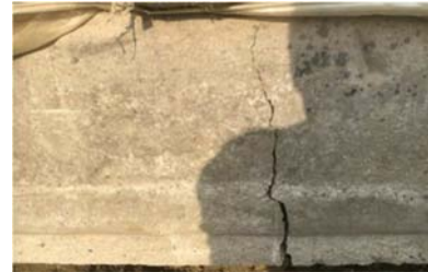
Figure 12. RC plate mid-span crack.
