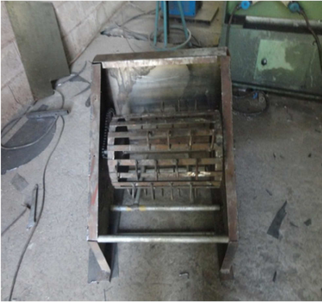
Figure 2. Modified threshing drum.
