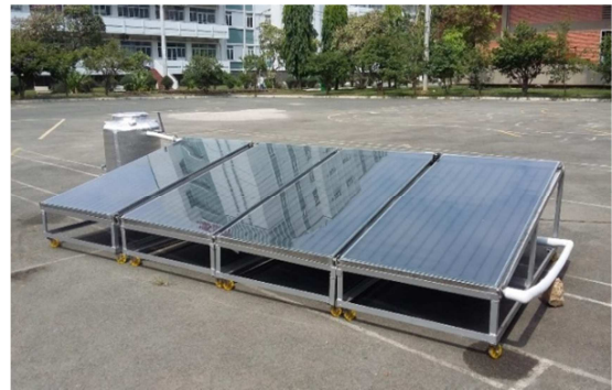
Figure 1. Schematic diagram of the solar flat-plate collector domestic hot water system with the constant flow rate in collectors loop.
