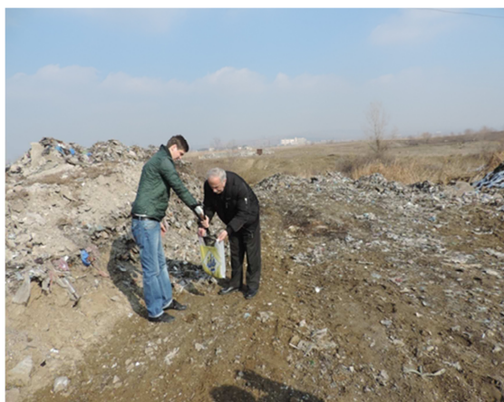
Fig. 3. The Soil Tests Gathered According to ISO 10381-1 and 10381-2.
