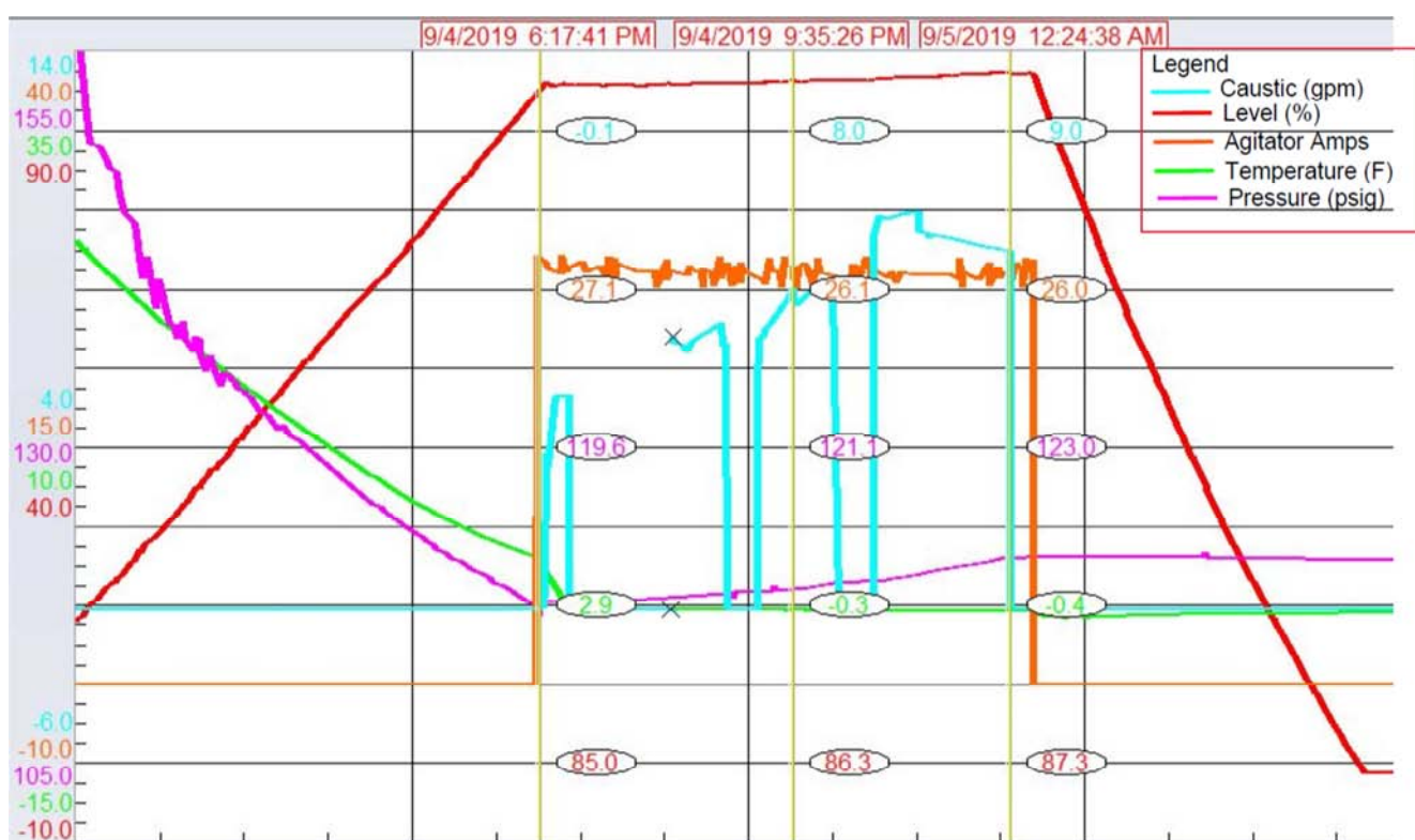
Figure 4. Aspen trend of final reactor used for MeCl elimination process before draining out to closed sump.
