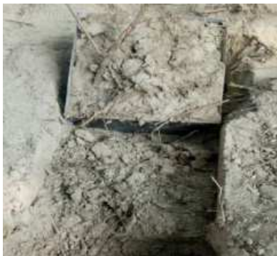
Figure 5. Failure plane of soil block with root.
