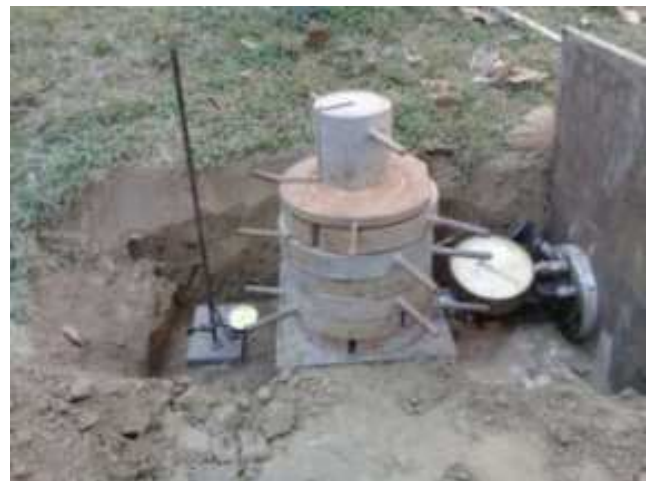
Figure 3. Experimental setup of in-situ direct shear test.
