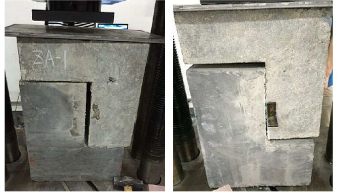
Figure 4. Fracture diagram of Z-type specimen.
