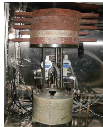
Figure 2. Loading system used in the frost heaving experiment.
