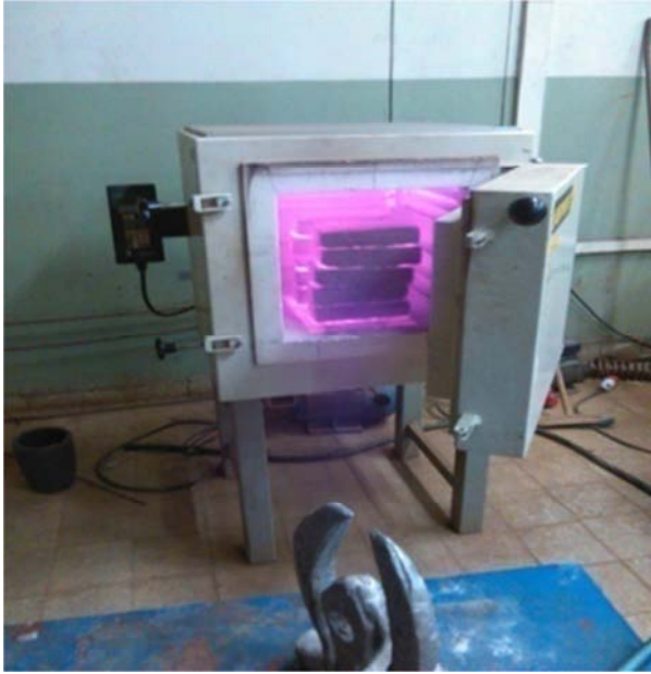
Fig. 3. Firing brick samples in a furnace.
