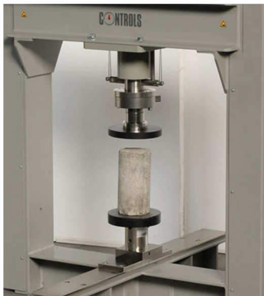
Figure 1. View of compressive loading system.
