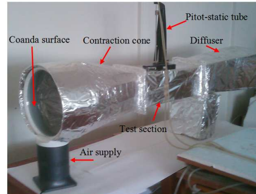
Fig 2. Test rig of mini-wind tunnel.
