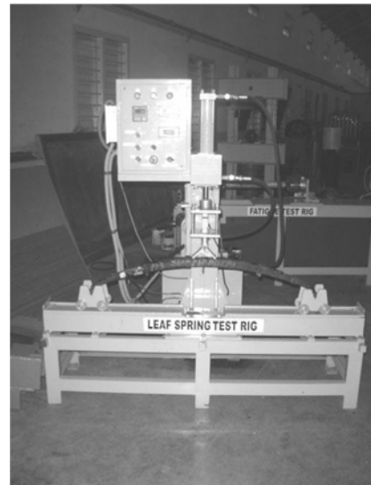
Figure 1. Static load test for steel leaf spring.
