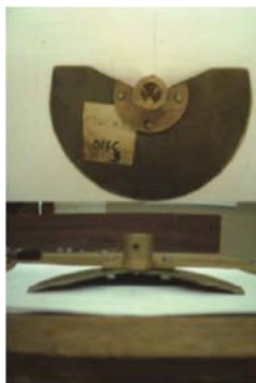
Figure 7. Rotating disc with cut-out.
