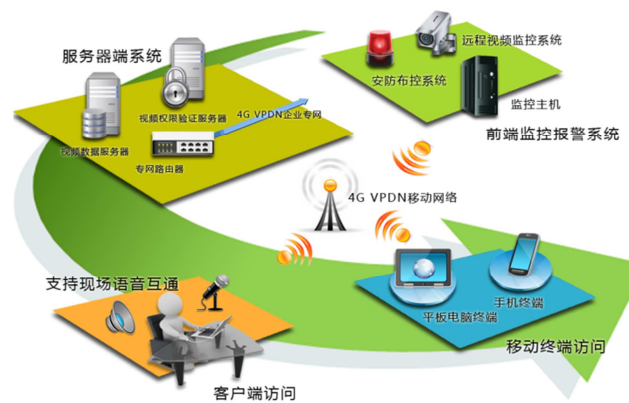
Fig. 1. Remote Monitoring System Configuration.
