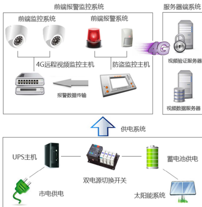
Fig. 2. Configuration of the Safety and Power Supply System.
