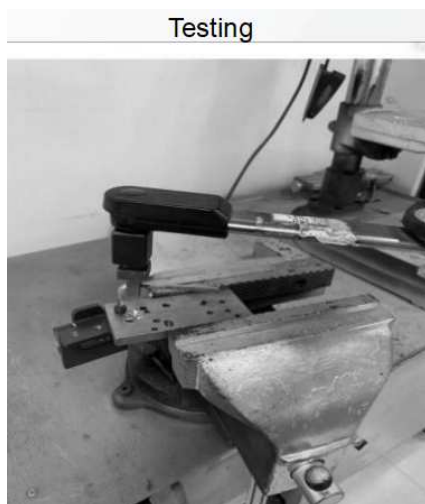
Figure 9. Torsion test of hinge.
