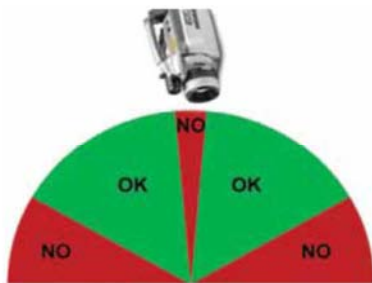
Figure 2. Correct viewing angles of PV panels during thermographic inspection proposed by manufacturing companies of thermographic equipment.
